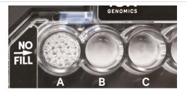
Recovery well A indicates a wetting failure. Not all wetting failures may present themselves with excess bubbles (foam).
