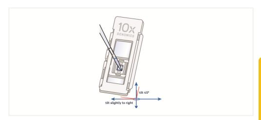
**f.** Add **100**  $\mu$ l 0.1 N HCl along the side of the wells to uniformly cover tissue sections, without introducing bubbles. Tap cassette gently to ensure uniform coverage.
