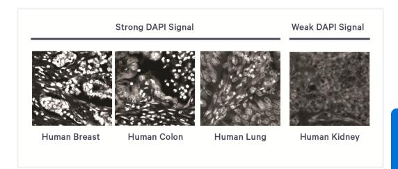
Sections with poor DAPI staining are unlikely to generate good data. All samples in the images below were imaged under the same conditions (405 nm channel). After evaluating DAPI staining, remove coverslip as described in 3.6 Coverslip Removal on page 65 and proceed to 2.5 Optional H&E Staining for Tissue Morphology Assessment below.
