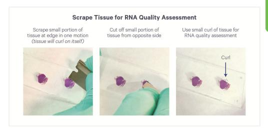
• Lift the curl using the blade, and use a clean pipette tip to transfer curl to one RNase-free 0.2-ml tube in a tube strip on ice. Store at -80°C for longterm storage or proceed immediately to RNA Extraction. If processing multiple archived slides, curls can be kept in tube strips on ice until ready for RNA extraction.
