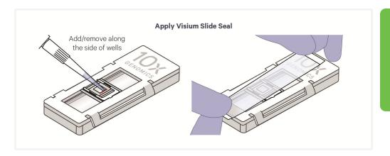
i. Remove slide seal. and using a pipette, remove all the HCl from the well corners.
