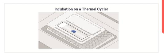
**c.** Remove slides from the oven or thermal cycler and allow to cool down to room temperature for **5 min**.
