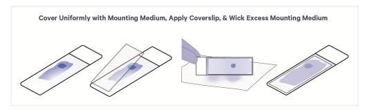
**e.** Remove any large excess of Mounting Medium by carefully wicking away from the edge of the coverslip using a lint-free laboratory wipe. Do not
