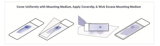
**d.** Remove any large excess of Mounting Medium by carefully wicking away from the edge of the coverslip using a lint-free laboratory wipe. Do not move coverslip and disturb tissue.
