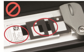
Slide is Broken due to Improper Loading
