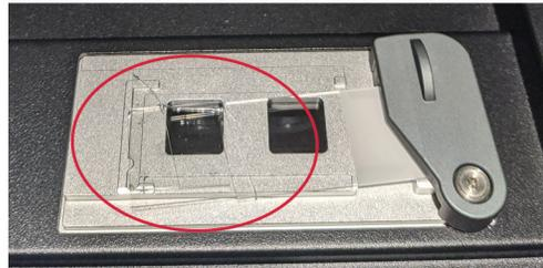
In the event of slide breakage, remove all traces of broken glass to avoid damaging the instrument. Exercise caution when removing glass to prevent injury.
