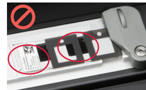
Slide is Broken due to Improper Loading
