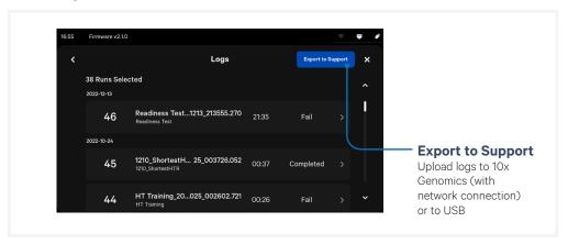
Idle time data are only instrument-specific logs that are not related to runs. The data can be exported during First-Time Use (FTU) setup by using the help icon on the top right corner of the screen. If the instrument is not performing a run, it can also be exported by navigating to Menu > System > Help and pressing "Send System Logs to Technical Support".
