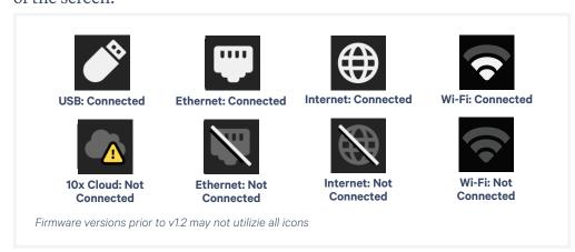
Click Diagnostics to enhance instrument stability and reliability. This enables the automatic transmission of diagnostic data, such as sensor readings, metrics, and user-editable fields to 10x Cloud when connected to the internet. To maximize internet stability and enable the 10x Genomics support team to quickly respond to issues, Diagnostics is enabled after software updates.
