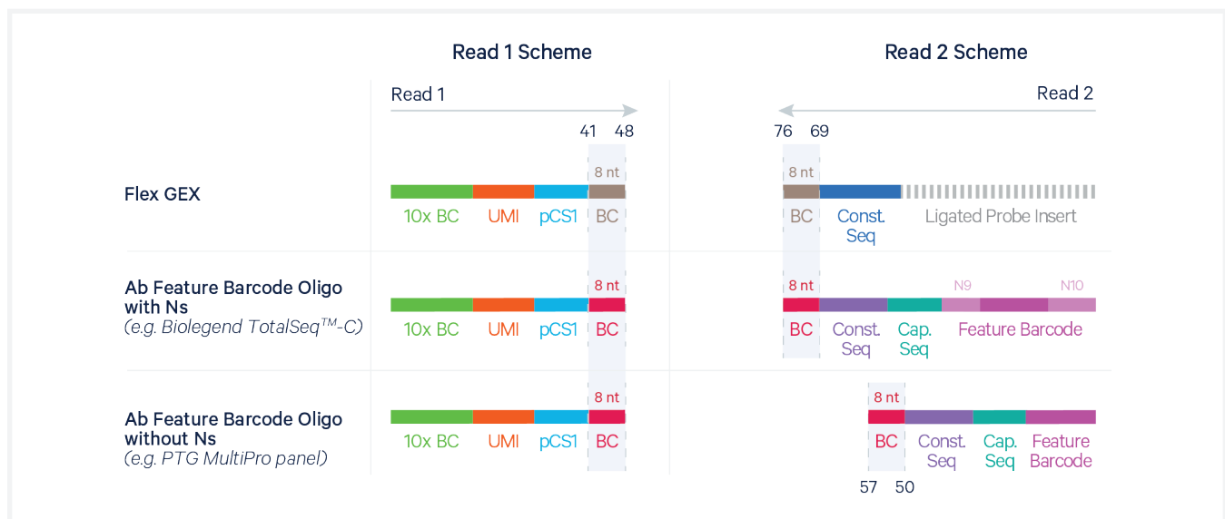
Figure 3. The location of the multiplexing Probe Barcode sequence in Read 1 versus Read 2 of Flex Gene Expression and two Flex Protein Expression libraries (BioLegend barcode oligo capture and PTG).
