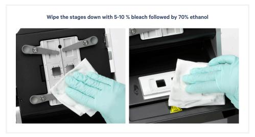
**d.** Close the lid (clicking sound indicates closure). Wipe down the base and lid of the instrument.
