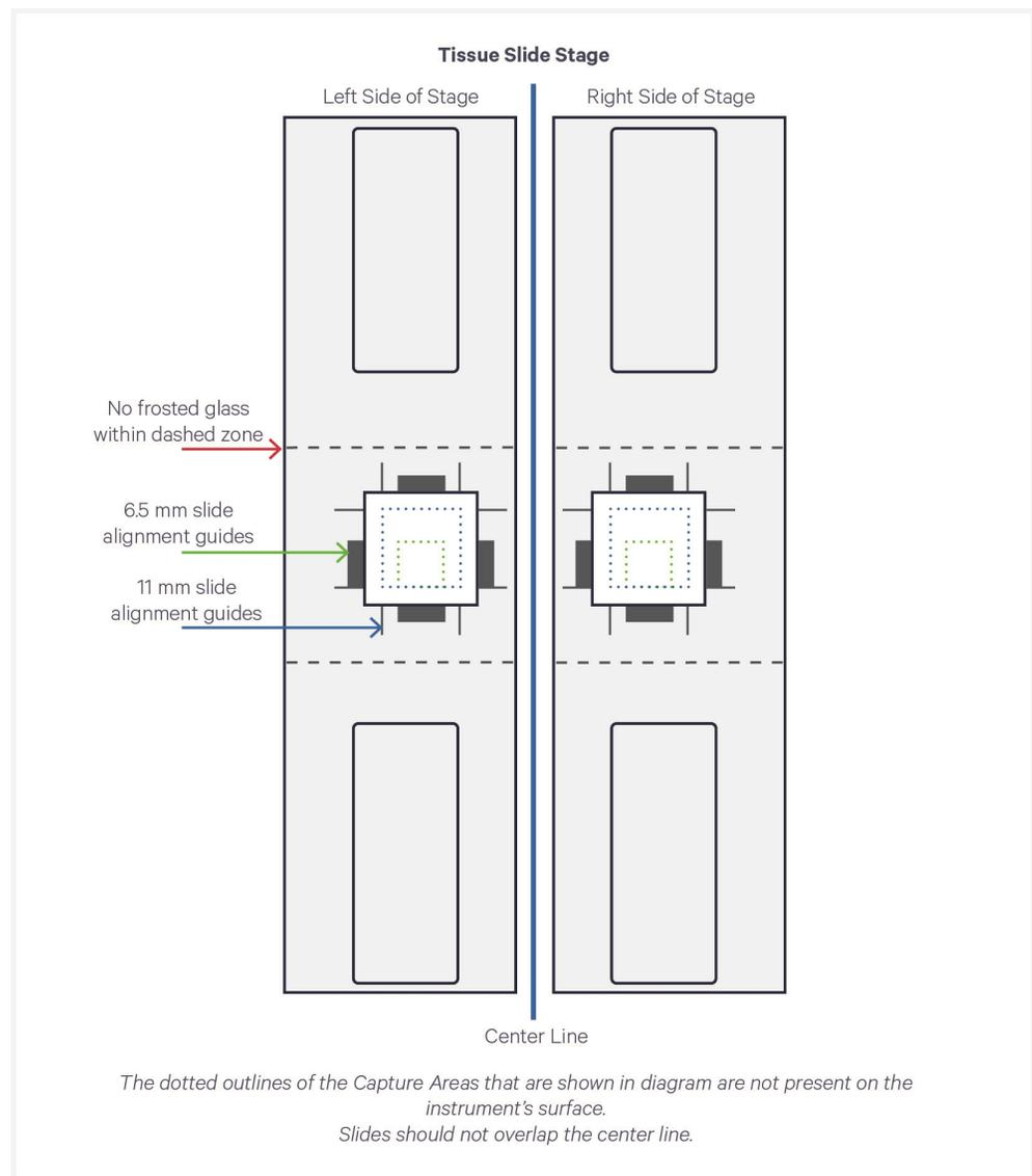
The **outside** of the alignment guides, shown in red, mark the inner boundaries of the fiducial frame on a Capture Area. They mark a distance **approximately** 6 mm (6.5 mm slides) or 10.5 mm (11 mm slides) wide on each side and surround the target region ensured to align within the fiducial frame. Though the Visium CytAssist instrument displays guides for 11 mm Capture Areas, the Visium HD Spatial Gene Expression Assay is only compatible with 6.5 mm Capture Areas.
