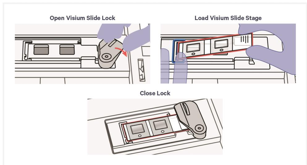
**Visium Slide Stage is Loaded Correctly with One Slide**
