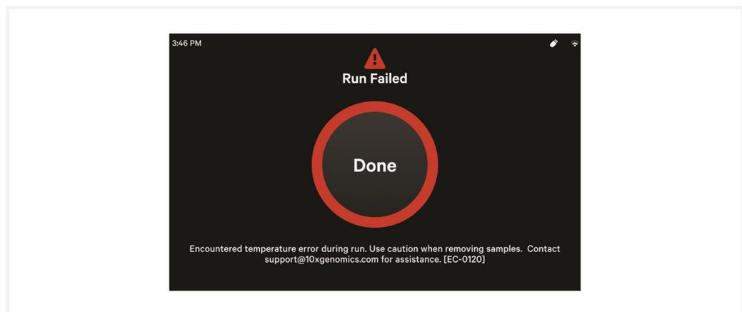
If the Visium CytAssist instrument overheats during an experiment run, the run will fail. A warning message will appear instructing users to carefully remove slides and contact [support@10xgenomics.com](mailto:support@10xgenomics.com).
