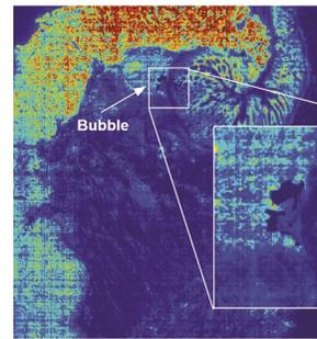
Bubbles during a sample run are rare, but may result in a lack of useable reads in the tissue area where the bubbled occurred. The most common cause of bubbles is incomplete drying of the tissue slide and/or the Visium HD slide. Bubbles can also result from inaccurate dispensing volume of Probe Release Mix. Ensure that the entire well is inspected for bubbles, not just the Capture Area. Ensure that the entire well is also dry during the drying step, not just the Capture Area.
