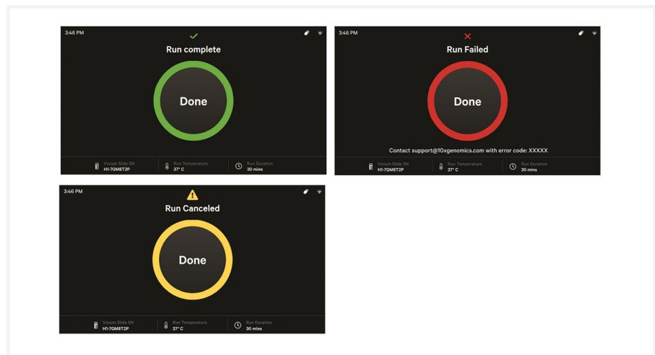
**aj.** Click "Done" button and open lid. **DO NOT** power off the instrument at this time, as it needs to process support data. It is normal for the Visium slide to move after opening instrument.
