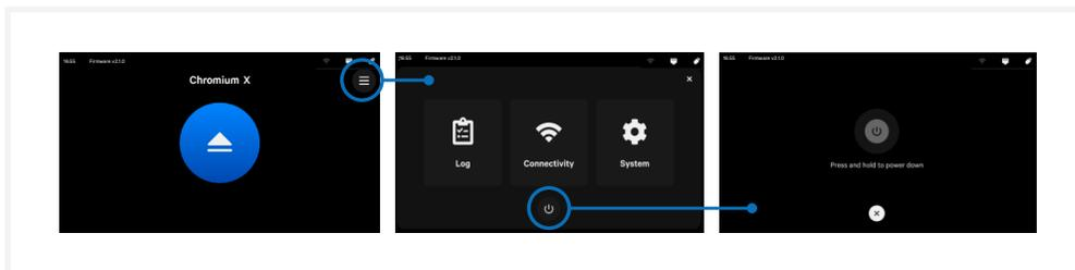
Power off the instrument by first performing a soft power down, by holding the power icon at the bottom of the menu options screen. In the soft power down mode, the screen will dim and display the time and the name of the instrument. To complete the shut down process, flip the power switch at the back.
