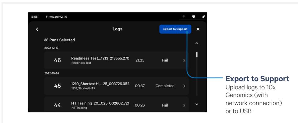
Idle time data are only instrument-specific logs that are not related to runs. The data can be exported during First-Time Use (FTU) setup by using the help icon on the top right corner of the screen. If the instrument is not performing a run, it can also be exported by navigating to Menu > System > Help and pressing “Send System Logs to Technical Support”.
