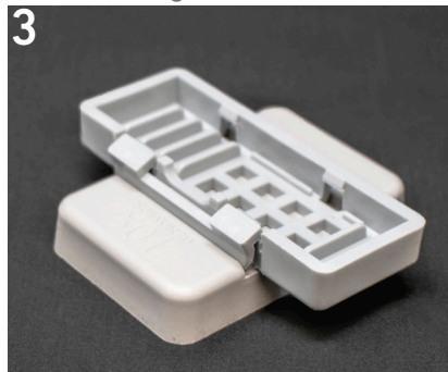
Visium Slide Cassette secured on alignment tool
