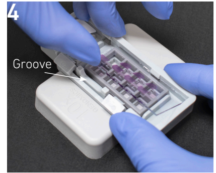
Lift slide at Visium Slide Cassette groove
