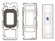
Place Xenium slide with label at bottom and tissue facing up into bottom half of cassette. Slip slide under slide clip located at bottom right of cassette.
