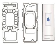
**3** Press slide down into grooves of the bottom half of the cassette until it sits firmly in place.
