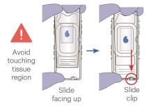
3 After slide is safely underneath slide clip, place opposite side down into carrier. Ensure slide is sitting flat.
