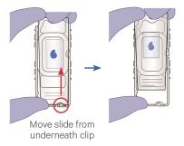
2 Open cassette by continuing to lift inner clips of top cassette upward.
