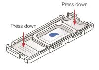
5 Apply even pressure on top of cassette until all clips click shut. Verify that clips are completely secured over tabs.
