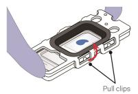
3 Hold top of slide and slowly lift slide out from underneath the slide clip. Then slowly remove from bottom cassette
