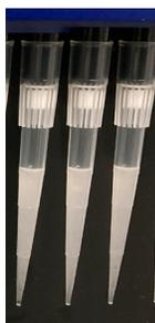
All liquid levels are similar in volume and opacity without air trapped in the pipette tips.
