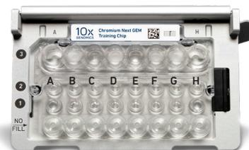
Recovery well G indicates a reagent clog. Recovery well C and E indicate a wetting failure. Recovery wells B, D, and F are normal. Wells A and H contain Surrogate Fluid.
