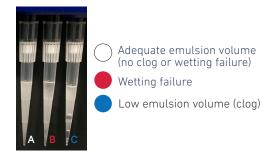
Pipette tip A shows normal GEM generation, pipette tip B indicates a wetting failure, and pipette tip C shows a clog and wetting failure.
