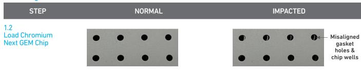
Gasket holes are aligned with the sample and gel bead wells.
