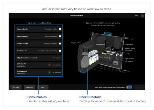
To aid in efficient and complete loading, the status of each item is shown on the left side of the screen and its location within the instrument deck is depicted on the right.
