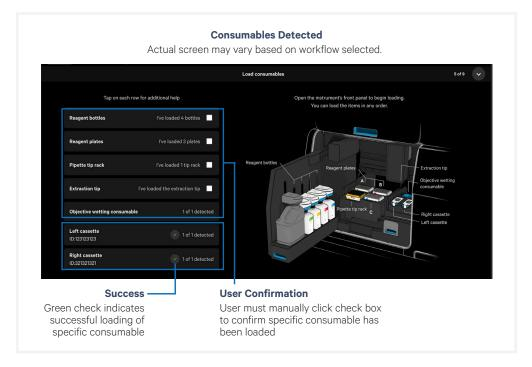
On the touchscreen, visually and manually confirm all consumables are loaded correctly and click "Continue". Close the instrument front panel.
