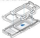
6 Add 100 µl PBS-T to cover the slide before loading onto the instrument
