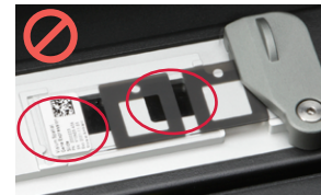
Slide is Broken due to Improper Loading
