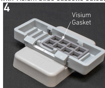
Press slide down until it is flush with the Visium Gasket and under tabs 3 & 4
