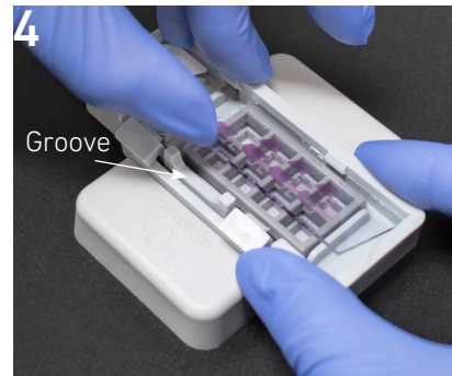
Lift slide at Visium Slide Cassette groove
