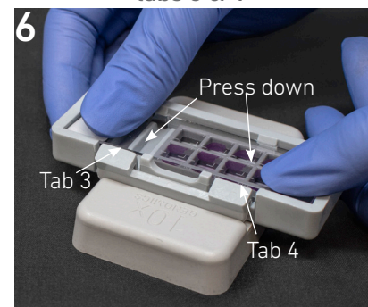
Press slide down until it is flush with the Visium Gasket and under tabs 3 & 4
