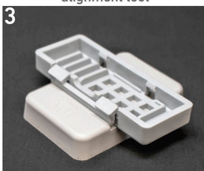
Visium Slide Cassette secured on alignment tool
