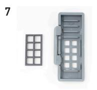
Mark the top portion of the Visium Gasket that faced the slide with an alcohol resistant marker
