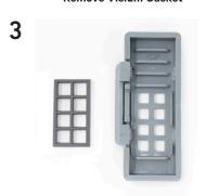
Spray with 70% isopropanol, then rinse with ultrapure water
