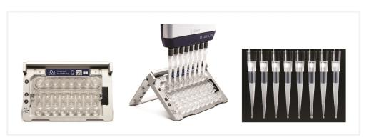
g. Over the course of ~20 sec, dispense GEMs into the tube strip on ice with the pipette tips against the sidewalls of the tubes.
