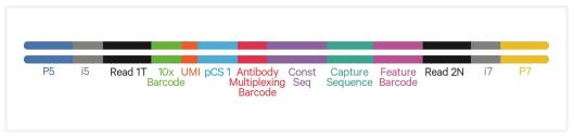
TruSeq Read 1 (Read 1T) and Nextera Read 2 (Read 2N) are used for pairedend sequencing of Fixed RNA – Protein Expression library. Read 2 sequences the Feature Barcode sequence, constant sequence, and Antibody Multiplexing Barcode that identifies the sample.
