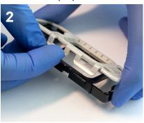
Pull inner clips from inner tabs to detach top and bottom halves of cassette
