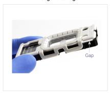
Open cassette by continuing to lift inner clips upward
