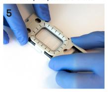
Place Xenium slide with tissue side facing upwards into bottom half of cassette; ensure label is toward bottom of cassette
