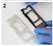
Secure clips of top half with tabs of bottom half (on both sides)
