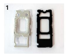
Press slide down into grooves of the bottom half of the cassette until it sits firmly in place
