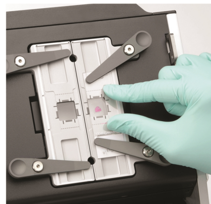
Adjust Tissue Slides to Match Alignment Guides
