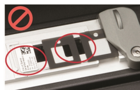
Slide is Broken due to Improper Loading
