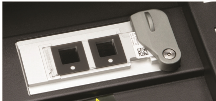
Visium Slide Stage is Loaded Correctly with One Slide
