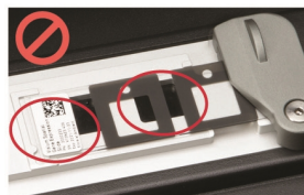
Slide is Broken due to Improper Loading
