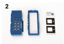
Place Visium slide with active surface facing upwards into lower half of cassette; ensure label is toward hinges
