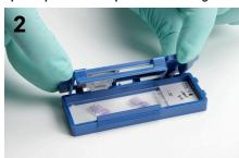
Hold slide by the label and lift slide out from lower half
