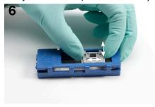
Turn cassette over and verify tissue area of interest is within gasket. DO NOT move gasket once cassette is closed. If necessary, open cassette and recenter gasket.
