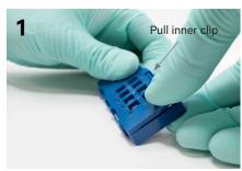
Open cassette by continuing to lift inner clip upward
