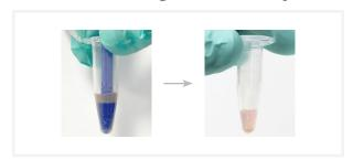
Grasp the pestle between the thumb and fingers and rotate the pestle (clockwise and counterclockwise 10-20X) inside the tube and go up and down with the scrolls trapped between the wall of the tube and the pestle for dissociation or until the scroll is broken into similarly sized smaller pieces.
