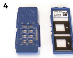
Secure outer clips of top half with outer tab of bottom half
