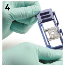
Adjust gasket such that gasket is over the tissue region of interest. The 6.5 mm gasket can be adjusted horizontally as well as vertically.
