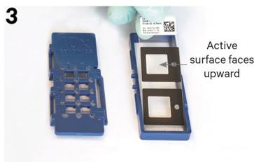
Press slide down into grooves of the bottom half of the cassette until it sits firmly in place
