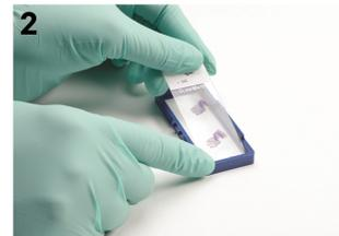
Securely combine gasket with top half of cassette until the gasket snaps into place.
