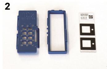
Place Visium slide with active surface facing upwards into lower half of cassette; ensure label is toward hinges
