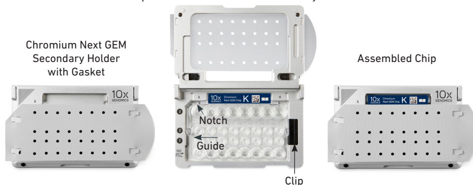
Chip in Chromium Next GEM Secondary Holder
