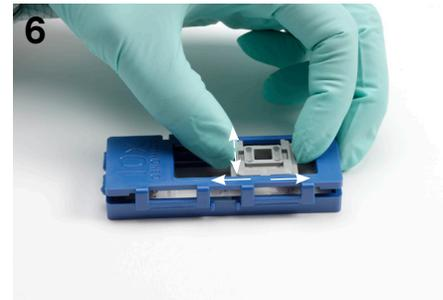
Turn cassette over and verify tissue area of interest is within gasket. DO NOT move gasket once cassette is closed. If necessary, open cassette and recenter gasket.
