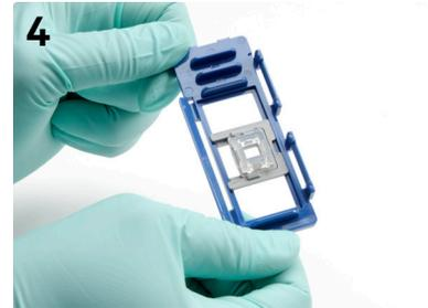
Adjust gasket such that gasket is over the tissue area of interest. The 6.5 mm gasket can be adjusted horizontally as well as vertically.
