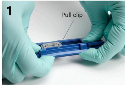
Open cassette by continuing to lift clip upward. If slide sticks to gasket, continue to apply even upward pressure to separate slide from gasket
