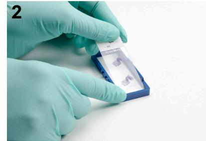
Securely combine gasket with top half of cassette until the gasket snaps into place.
