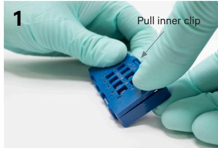
**Open cassette by continuing to lift inner clip upward**
