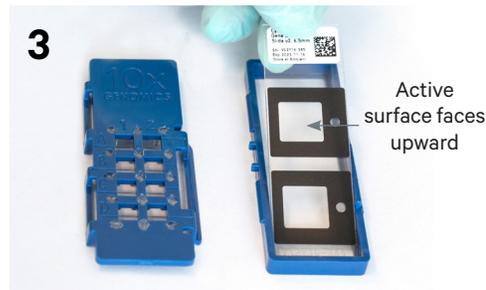
Press slide down into grooves of the bottom half of the cassette until it sits firmly in place
