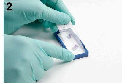
The 6.5 mm gasket can be adjusted horizontally and rotated in two directions (180°) while 11 mm gasket can be rotated in four directions (90°). Determine the appropriate configuration that allows the gasket to encompass the tissue area of interest.
