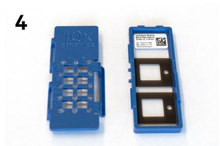
Secure outer clips of top half with outer tab of bottom half
