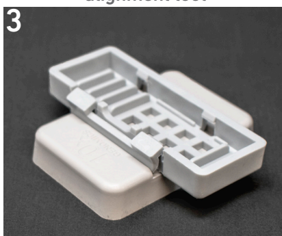
Visium Slide Cassette secured on alignment tool
