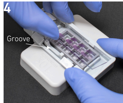
Lift slide at Visium Slide Cassette groove
