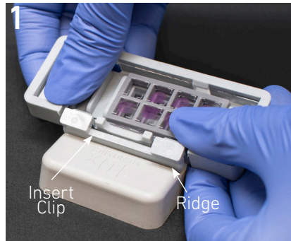
Position Visium Slide Cassette along alignment tool ridges
