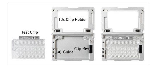
c) Close the hinged lid of the 10x Chip Holder. After loading the Test Chip, the 10x Chip Holder should lay flat on the bench top with the lid closed.
