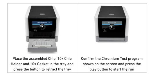
At the completion of the run (3 min), the Chromium Single Cell Controller will chime. Press the button to eject the tray. Remove and disassemble the Chip Holder assembly. Press the button again to retract the empty tray (or the tray will automatically close after 40 sec).
