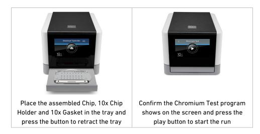
d) At the completion of the run (3 min), the Chromium Controller will chime. Press the button to eject the tray. Remove and disassemble the Chip Holder assembly. Press the button again to retract the empty tray.
