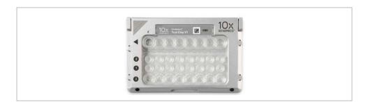
d) Orient the assembly so that the Partitioning Oil wells (row labeled 3) are toward you.
