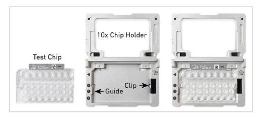
c) Close the hinged lid of the 10x Chip Holder. After loading the Test Chip, the 10x Chip Holder should lay flat on the bench top with the lid closed.
