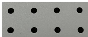
Gasket holes are aligned with the sample and gel bead wells.
