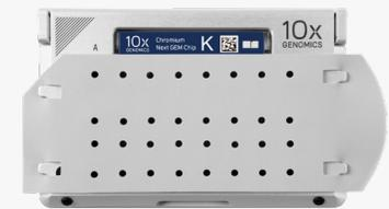
Keep horizontal to avoid wetting the gasket. **DO NOT** press down on the gasket.
