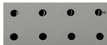
Misaligned gasket holes & chip wells
