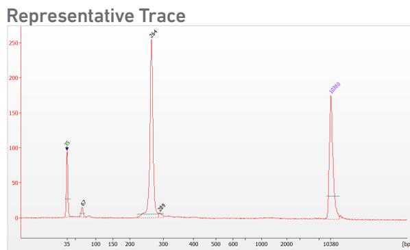
Select the region between 200-400 bp to determine the average fragment size from the Bioanalyzer trace. This will be used as the insert size for library quantification.
