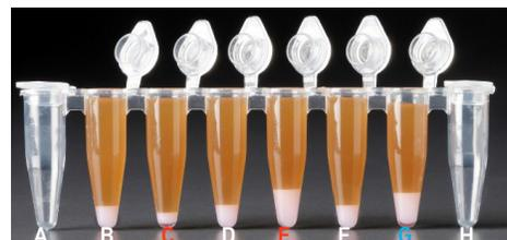
Tube **G** indicates a reagent clog has occurred. There is an abnormal ratio of Dynabeads Cleanup Mix (brown) to Recovery Agent/Partitioning Oil (appears white).
