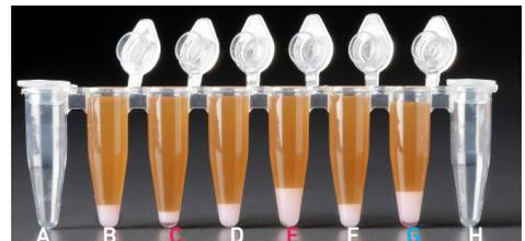
Tube **G** indicates a reagent clog has occurred. There is an abnormal ratio of Dynabeads Cleanup Mix (brown) to Recovery Agent/Partitioning Oil (appears white).
