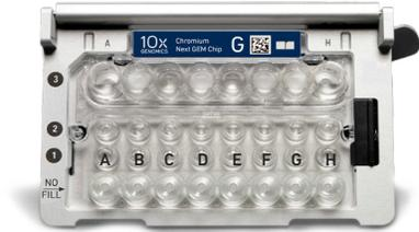
Recovery well G indicates a reagent clog. Recovery well C and E indicate a wetting failure. Recovery wells B, D, and F are normal. Wells A and H contain 50% Glycerol Solution.
