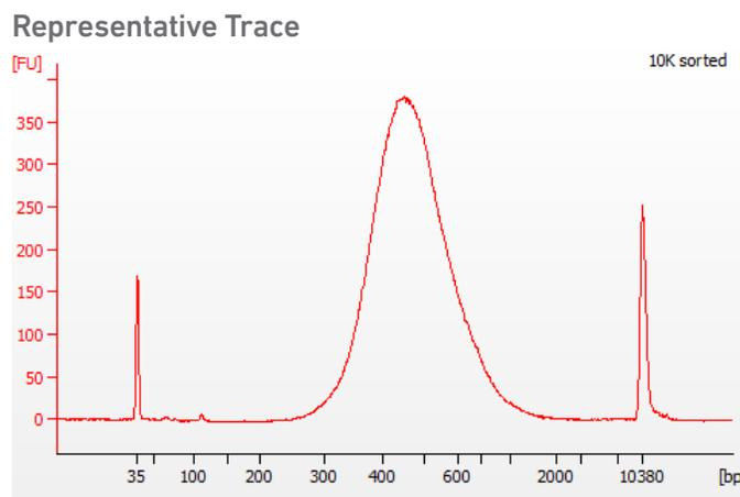
Select the region between 200-2,000 bp to determine the average fragment size from the Bioanalyzer trace. This will be used as the insert size for library quantification.
