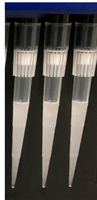
All liquid levels are similar in volume and opacity without air trapped in the pipette tips.
