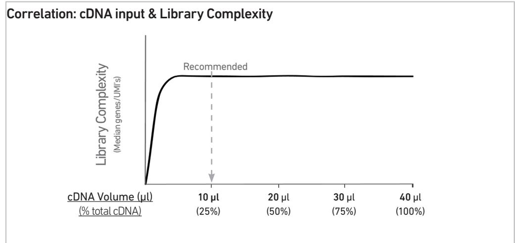
Note that irrespective of the total cDNA yield (ng), which may vary based on cell type, targeted cell recovery etc., this protocol has been optimized for a broad range of input mass (ng), as shown in the example below. The total number of SI PCR cycles (step 3.5e) should be optimized based on carrying forward a fixed proportion (10  $\mu$ l, 25%) of the total cDNA yield calculated during Post cDNA Amplification QC & Quantification (step 2.4).
