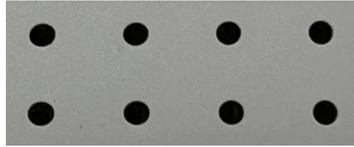
Gasket holes are aligned with the sample and gel bead wells.
