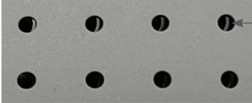
Misaligned gasket holes & chip wells |
