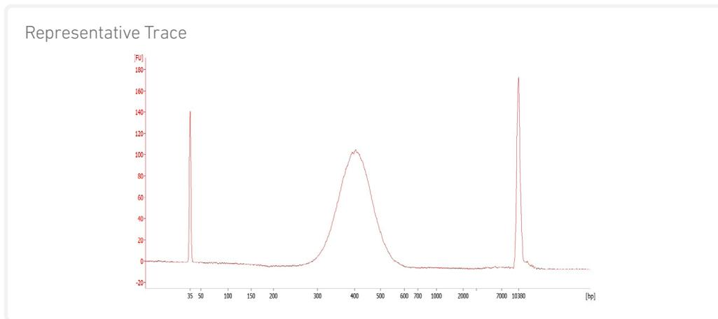
Select the region between 200-2,000 bp to determine the average fragment size from the Bioanalyzer trace. This will be used as the insert size for library quantification.
