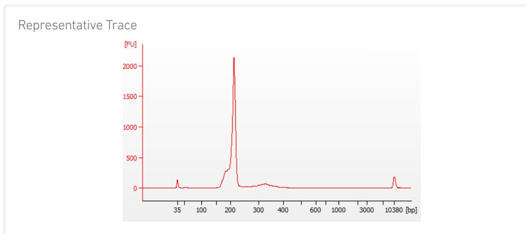
Select the region between 150-300 bp to determine the average fragment size from the Bioanalyzer trace. This will be used as the insert size for library quantification.
