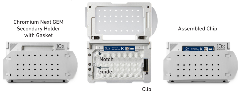
Chip in Chromium Next GEM Secondary Holder
